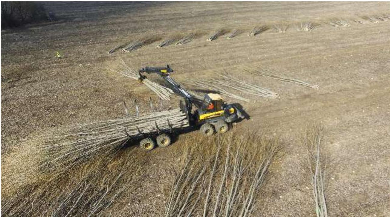
*Figure 56 Photo of large forwarder used for on-field transport of prebundled whole trees*
