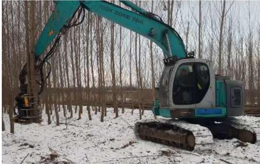
*Figure 55 Photo of tracked feller buncher harvester with shears*
