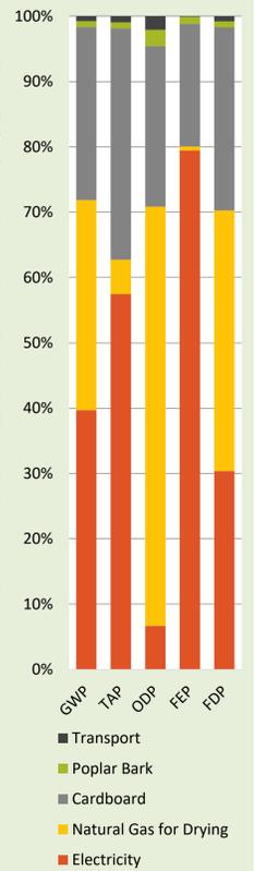
Figure 1: Contribution analysis for NBBM 2 in different impact categories
