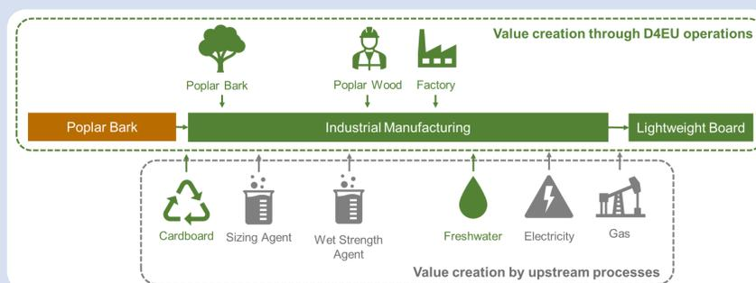
Figure 4: Processes considered for the value-added calculations
