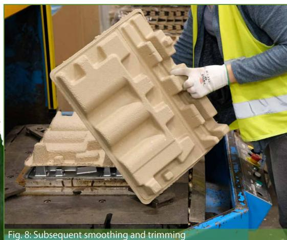
Fig. 8: Subsequent smoothing and trimming
