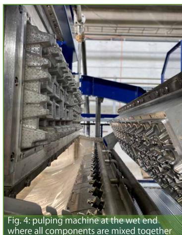
Fig. 4: pulping machine at the wet end where all components are mixed together
