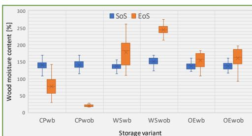
Fig. 3: Changes in moisture content for the 9 month storage period in 2018 (start of storage/SoS vs. end of storage/EoS)
