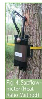
Fig. 4: Sapflowmeter (Heat Ratio Method)
