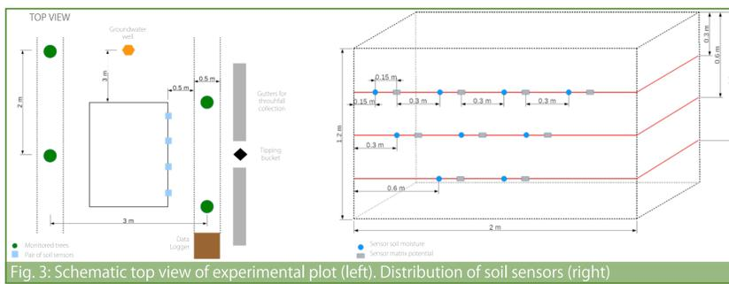
Fig. 3: Schematic top view of experimental plot (left). Distribution of soil sensors (right)
