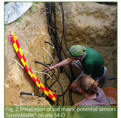
Fig. 2: Installation of soil matrix potential sensors TensioMARK® on site S4-D
