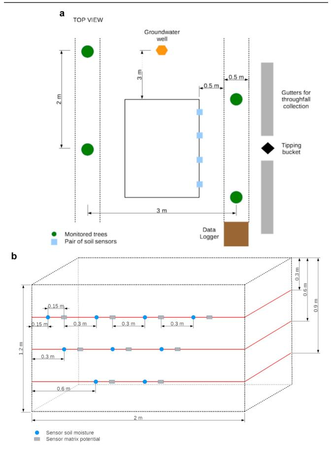
◄Fig. 2 a Schematic top view of the experimental plot, including monitored trees and groundwater well. b Distribution of sensors of soil moisture and matric potential in the soil profile pit at each site. At the site with low groundwater table (S4-D), the first sensor row was installed at 25-cm soil depth to avoid the limit with the next horizon. At the site with fluctuating groundwater level (S2-F), at 90-cm soil depth, high gravel content prevented the installation of matric potential sensors
