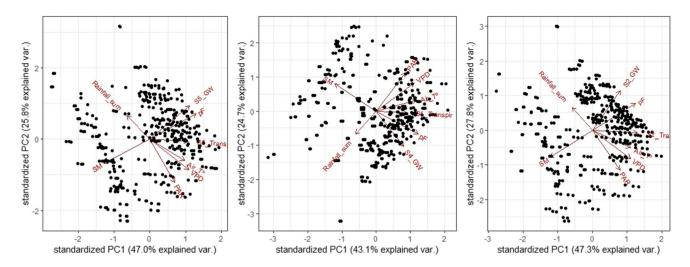
**Fig. 7** Results of principal component analysis (PCA) for the site with higher groundwater level (S5-N, left), for the site with low groundwater level (S4-D, center), and for the site with fluctuating groundwater level (S2-F, right) including variance per principal components (PC) 1 and 2. Analyzed variables included daily mean groundwater level (GW), daily median of all the sensors of soil mois-
