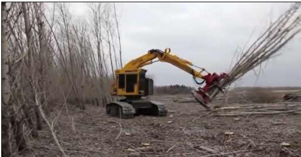
*Figure 39 Photo of tracked feller buncher harvester with hot disk harvesting a hybrid poplar plantation in Minnesota, USA.*
