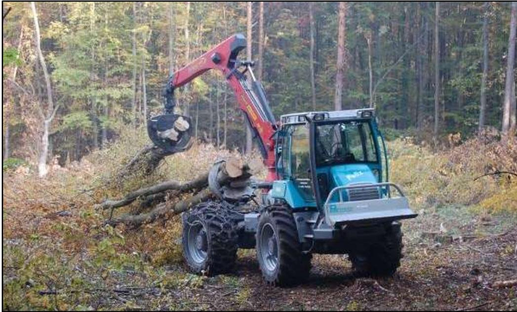
Figure 40 Photo of clambunk forwarder used for on-field transport of prebundled logs
