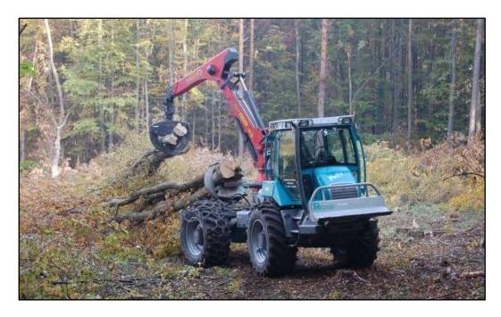
Figure 40 Photo of clambunk forwarder used for on-field transport of prebundled logs
