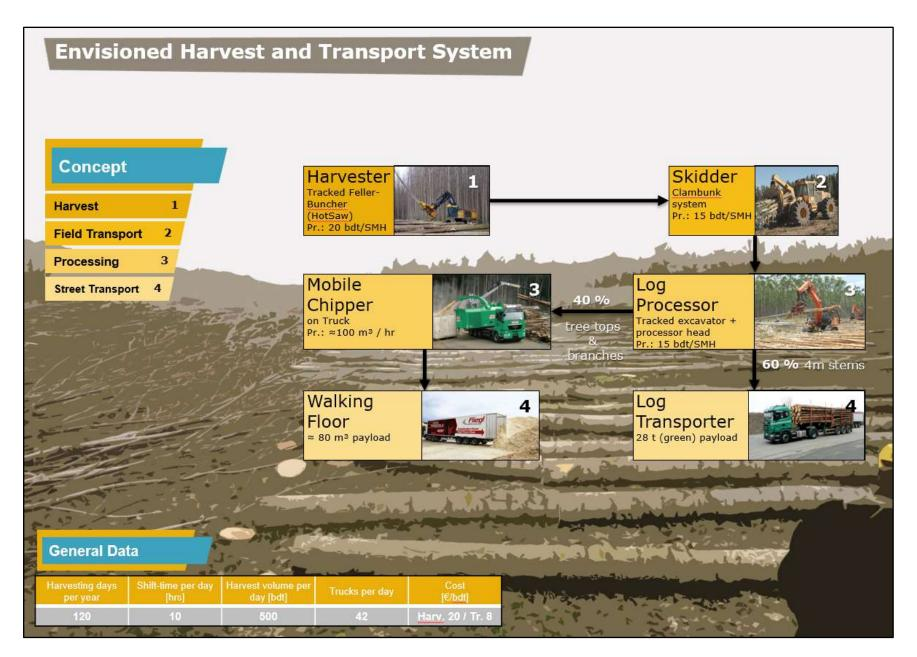
Figure 42 Diagram and summary data of envisioned harvest and log processing concept for the SRP project
