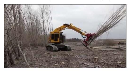
Figure 39 Photo of tracked feller buncher harvester with hot disk harvesting a hybrid poplar plantation in Minnesota, USA.
