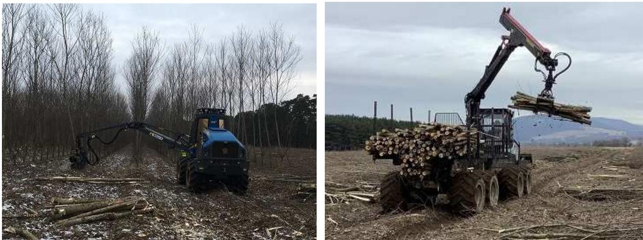
**Figure 1.** The harvester (left) and the forwarder (right) used for the experiment.
