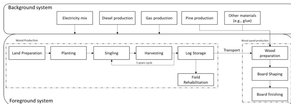
**Figure 1.** Summary of system boundaries for the case study of wood panel boards.
