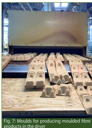
Fig. 7: Moulds for producing moulded fibre products in the dryer
