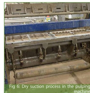
Fig 6: Dry suction process in the pulping machine
