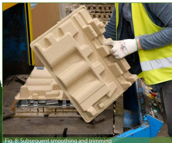
Fig. 8: Subsequent smoothing and trimming
