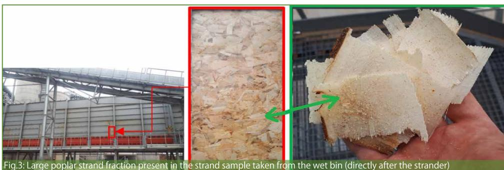
Fig.3: Large poplar strand fraction present in the strand sample taken from the wet bin (directly after the strander)
