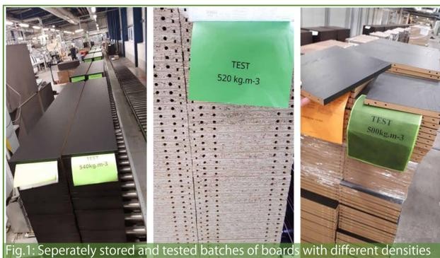
Fig.1: Separately stored and tested batches of boards with different densities
