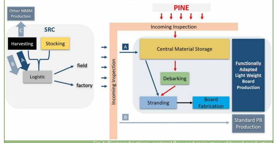
Fig.4: Biomass fractions, material flow and main steps of board production
