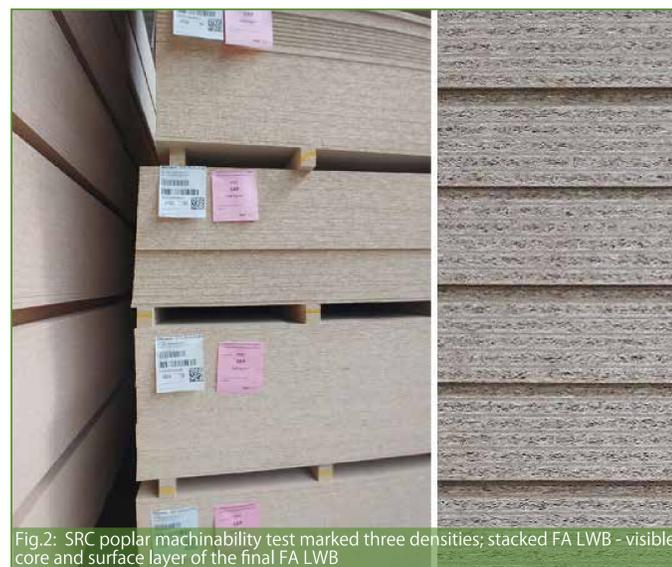
Fig.2: SRC poplar machinability test marked three densities; stacked FA LWB - visible core and surface layer of the final FA LWB
